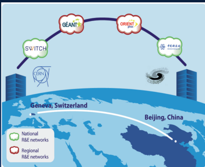
The route of data between IHEP and CERN via national and regional R&E networks/links
